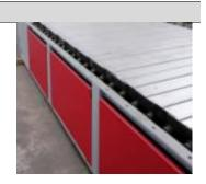
The chain is automatically lubricated on each side by a tank with manual opening
