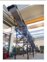
Removable protections for a fast inspection and maintenance of the belt.
