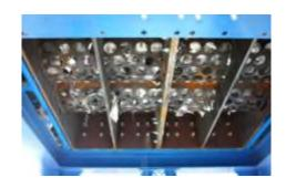
Blades locking with trapezoidal special thread and nuts that ensure the perfect tightening in any working conditions.
