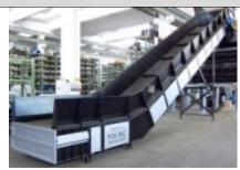
Removable protections for a fast inspection and maintenance of the belt
